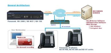
Reliable and secure call recording through SPAN (port Mirror) on the switch where the PBX is connected.
